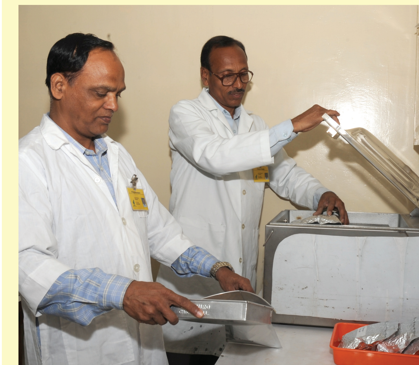
Vacuum sealing of seeds for long-term conservation and safety duplication.
