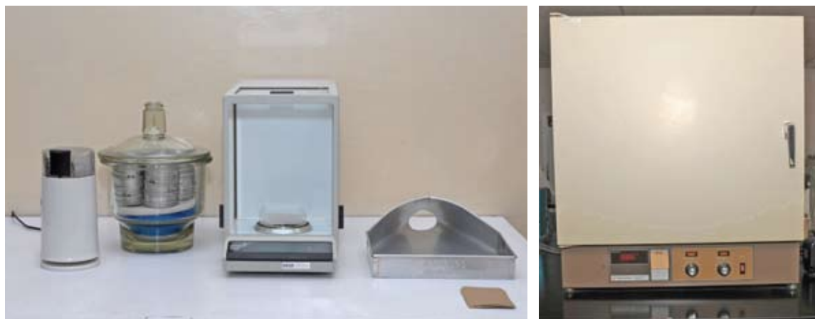
Figure 4B.2. Equipment used to determine seed moisture content.
