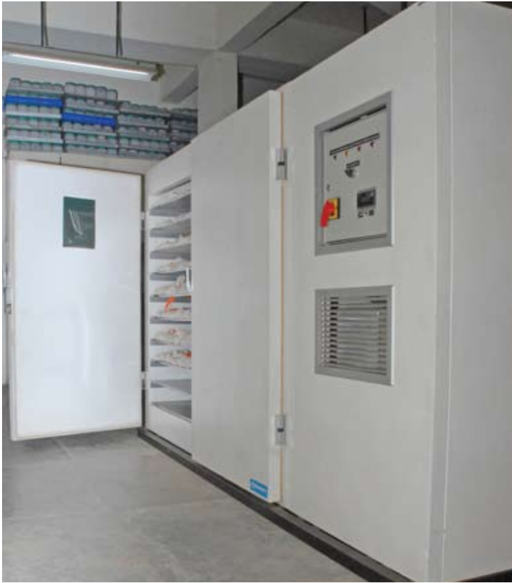
Figure 4C.1.1. Seed-drying cabinet at ICRISAT genebank.
