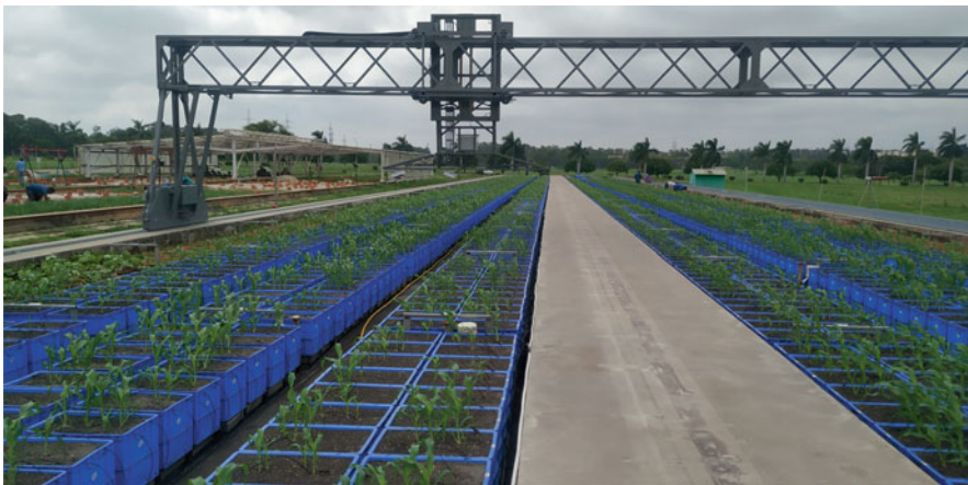
Fig. 7.3 LeasyScan: high-throughput phenotyping platform
